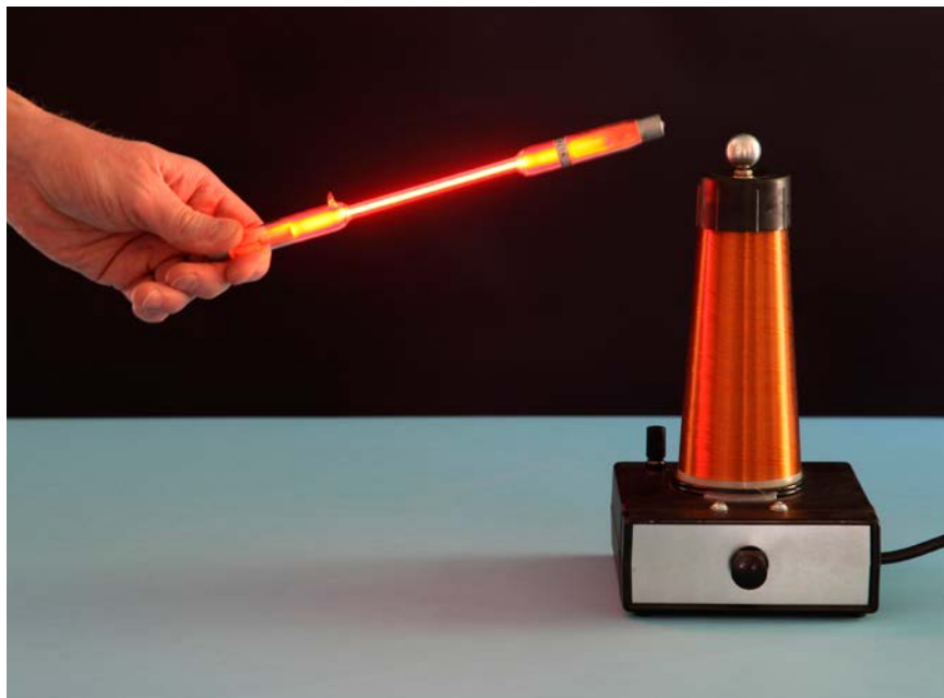
A modern Tesla coil sends electrical power through the air to light up a neon tube.
